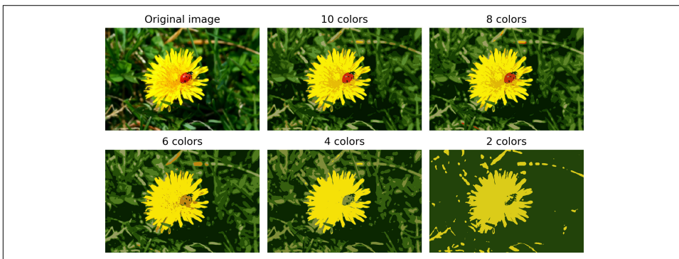
Figure 9-12. Image segmentation using K-Means with various numbers of color clusters
